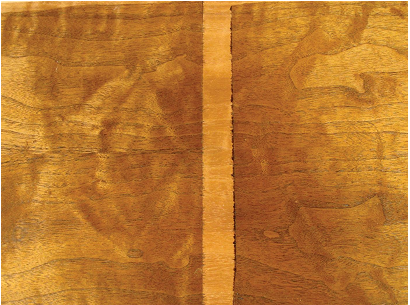
Blotching. Sanding to a very fine grit does not reduce blotching. I sanded the left side of this cherry panel to #400 grit and the right side to just #150 grit. The picture was difficult to take because of chatoyance, the reversal of the darker blotchy areas when you change your viewing angle. But the angle I used here shows an equivalent darkness on both sides.
